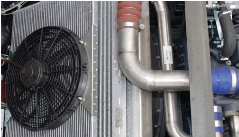
COOLING SYSTEM WITH DEUTZ ENGINE
