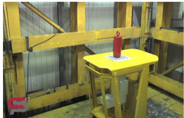
Fig. 5. FOPS test stand example [15]
