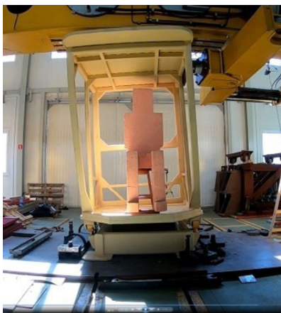
Fig. 19. ROPS structure under the lateral load
